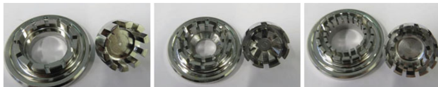
Fig. 11.7 Possible rotor–stator design to vary the shear and flow conditions in the mixing chamber
