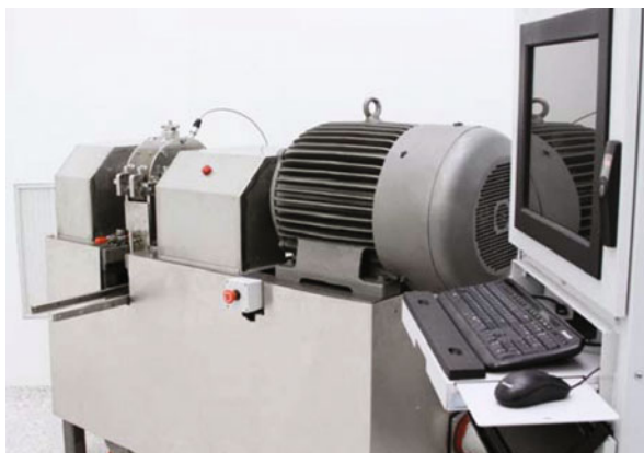
Fig. 18.1 Batch-mode GMP KinetiSol compounder model TC-254B
