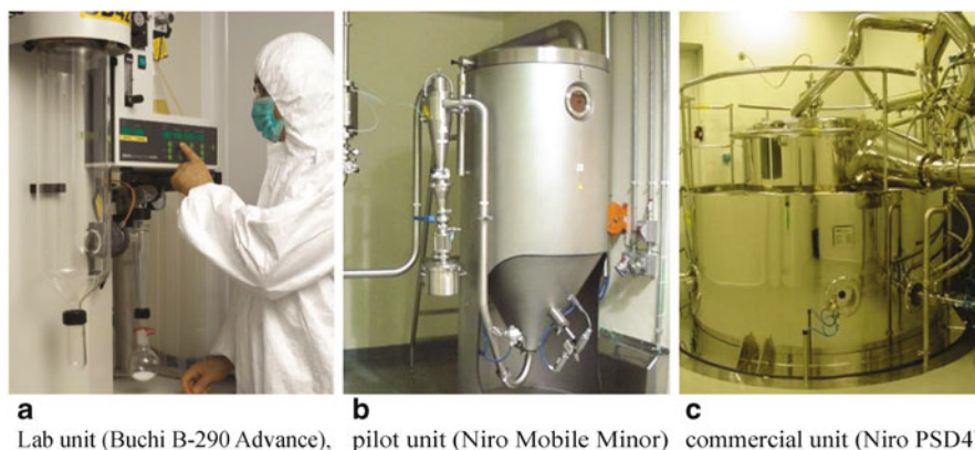
Fig. 8.1 Lab-, pilot-, and commercial-scale spray dryers at Hovione
