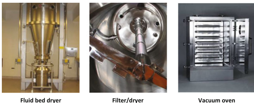
Fig. 11.10 Types of dryers commonly used in the MBP manufacturing
