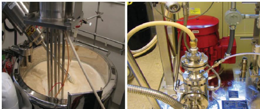
Fig. 10.4 MBP manufacture reactors showing batch mode reactor (left) and continuous mode reactor (right)
