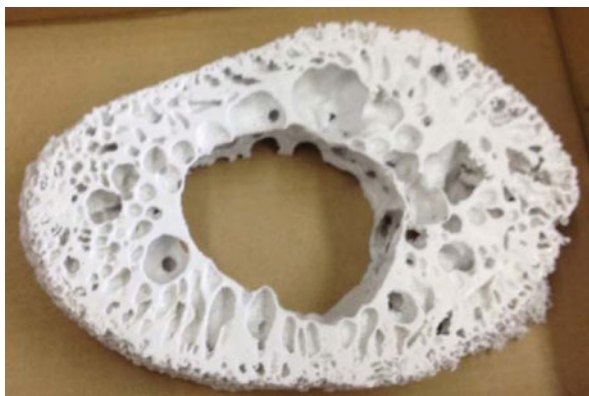
Fig. 10.6 Microstructure of MBP particle reproduced using 3D printing (courtesy of Dr. Siegfried Krimmer)
