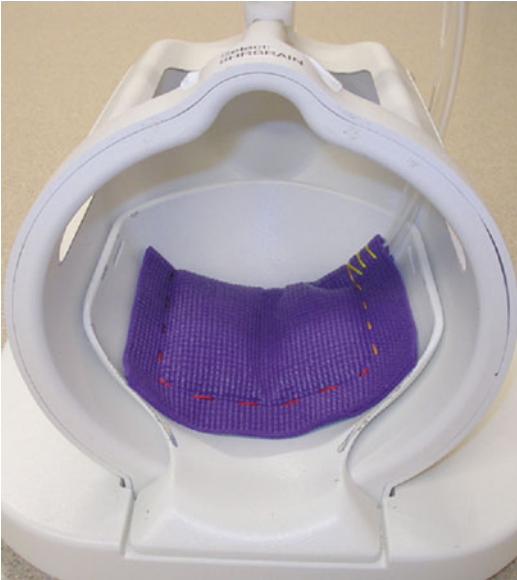
Fig. 8.1 Soft pillow driver used to introduce shear waves into the brain positioned within a standard eight channel head coil
