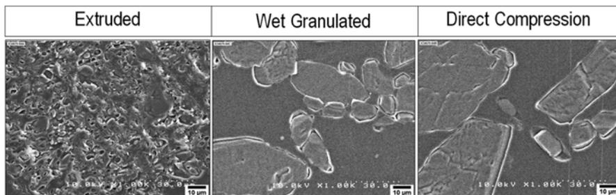
**Fig. 10.12** Porosity of metformin hydrochloride extruded granules. Scanning electron microscopy pictures of the cross section of granules embedded in epoxy resin indicate that granules made by the extrusion process had more internal voids relative to granules made by alternate processes. This may explain the lower granule density for those made by extrusion relative to those made by alternate process
