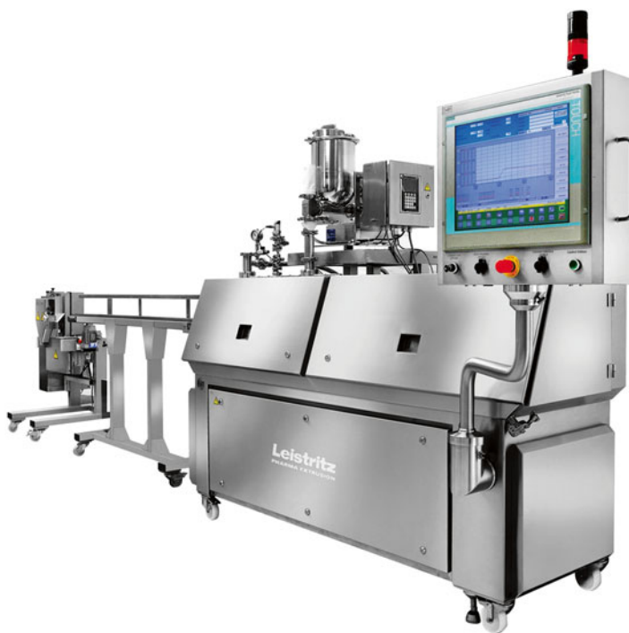
Fig. 10.1 Pilot-scale 18 mm Leistritz ZSE extruder as used in some of the work highlighted in this chapter (picture courtesy of Leistritz Extrusionstechnik/Germany)
