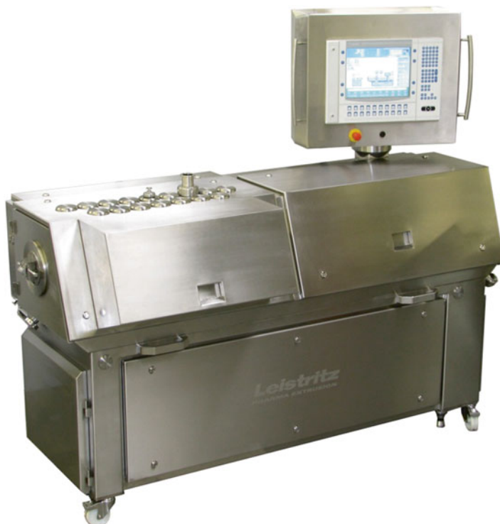
Fig. 10.2 Leistriz ZSE 18 PH extruder, 18 mm barrel diameter, suitable for GMP manufacturing (picture courtesy of Leistriz Extrusionstechnik/Germany)
