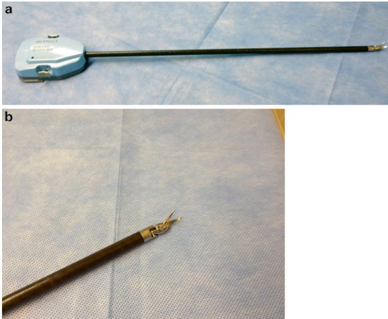
Fig. 2.25 (a) Da Vinci® robot curved scissors. (b) Tip of Da Vinci® robot curved scissors (Intuitive Surgical, Inc., Sunnyvale, CA)
