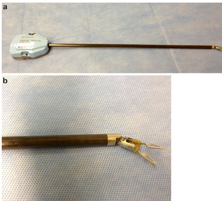
Fig. 2.23 (a) Da Vinci® robot precise bipolar forceps. (b) Tip of Da Vinci® robot precise bipolar forceps (Intuitive Surgical, Inc., Sunnyvale, CA)
