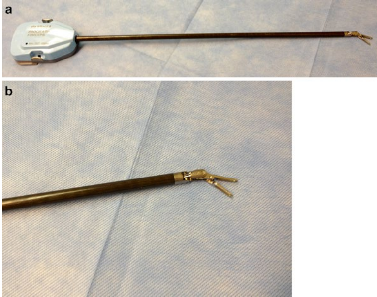
Fig. 2.24 (a). Da Vinci® robot prograsp forceps. (b) Tip of Da Vinci® robot prograsp forceps (Intuitive Surgical, Inc., Sunnyvale, CA)
