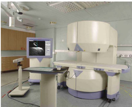
Fig. 16.3 Philips Medical Systems Open Configuration interventional MRI unit with in-room monitor, in-room workstation with imaging capability, and a foot pedal for the operator which controlled sequence start
