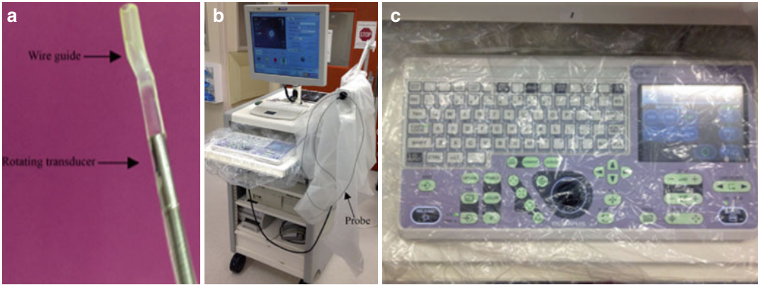
Fig. 12.1 ELUS probe and system. (a) Photograph of a 5.4 French (1.8 mm) ELUS probe. This probe can be passed over a guidewire, and it has a shielded transducer, which continuously rotates to provide radial images with adjustable scanning depths of 1–6 cm. (b) Photograph of the ELUS system setup at our institution. The actual system generator is hidden underneath the keyboard; a cable
