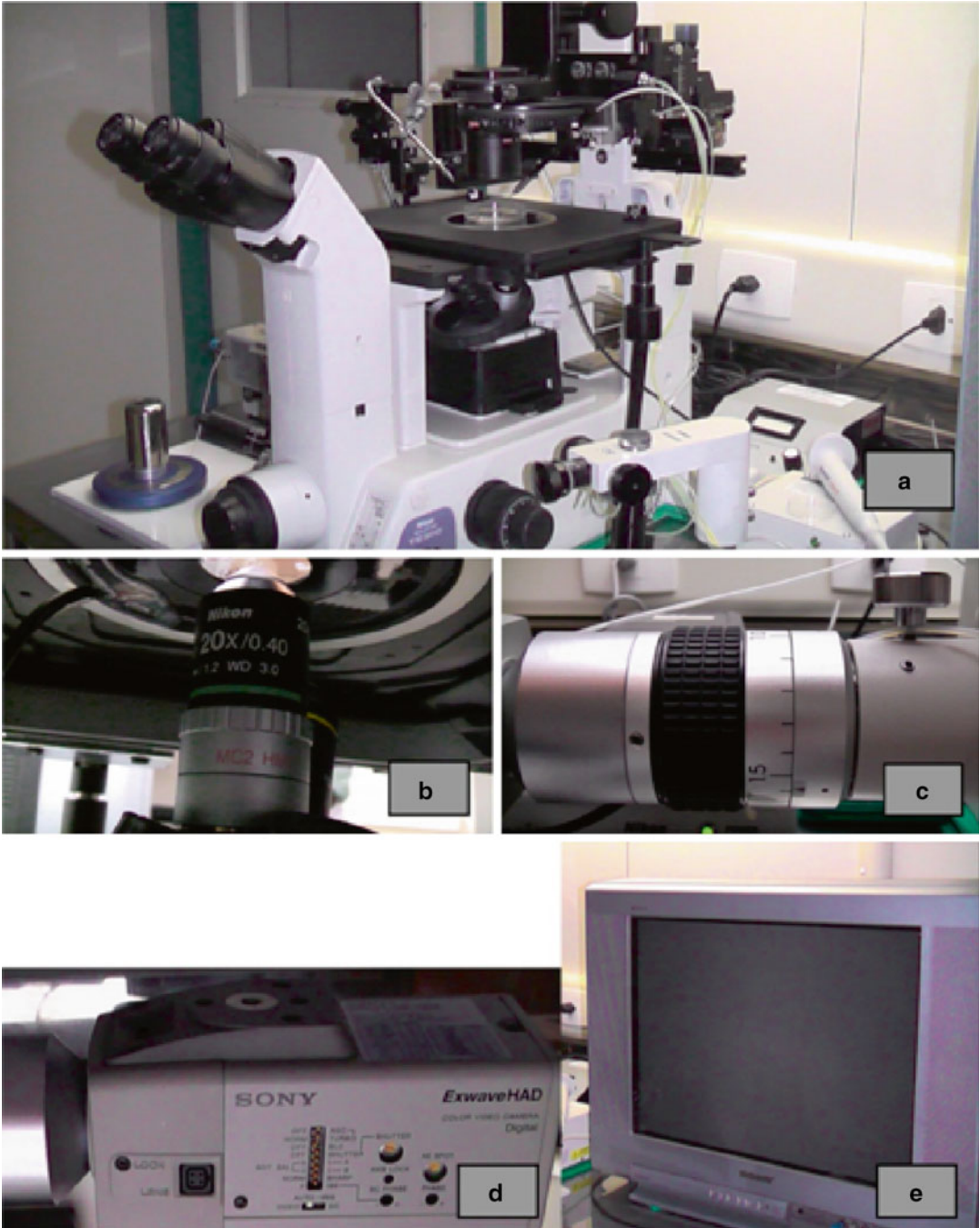
Fig. 8.1 (a) The polarization inverted microscope (TE 300 Nikon, Japan) equipped with Hoffman contrast and polarizing lens; (b) Hoffman objective of 20 \times ; (c) C-mount; (d) Camera; and (e) 21-inch monitor
