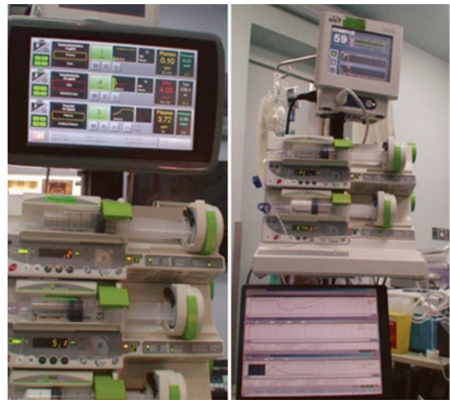
Figure 22.1 Left: Ez fusor. Right: Anestfusor. Both control infusion pumps (DPS, Fresenius Kabi)
