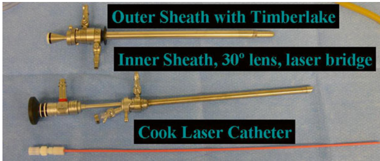
Fig. 17.3 The disassembled laser scope and protective laser catheter. The device shown is the Storz 28 Fr set consisting of a 28 Fr outer sheath, inner sheath with stabiliz-
