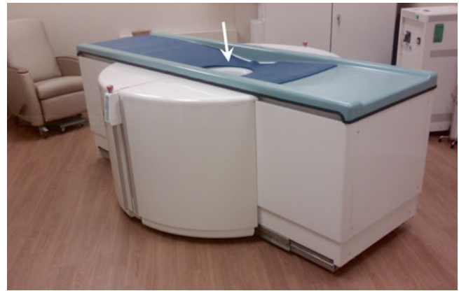
Fig. 19.8 Dedicated breast CT scanner. The patient lies prone and hangs breast in vertical gantry ( arrow ) (Courtesy of Ioannis Sechopoulos, PhD)
