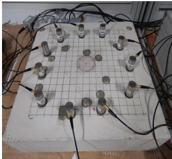
Fig. 4 Concrete sample without steel (sample 1)
