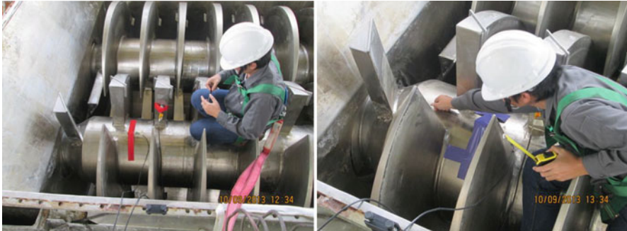
Fig. 11 AE testing for leakage and cracking of drum
