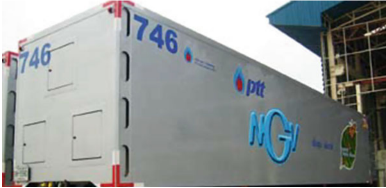
Fig. 4 Tube-trailer transport trucks
