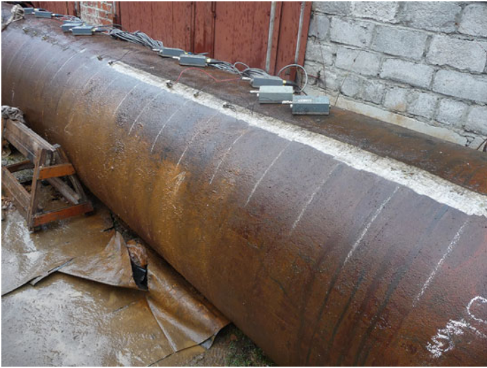
Fig. 7 A pipeline with the thickness profile in the form of the step function
