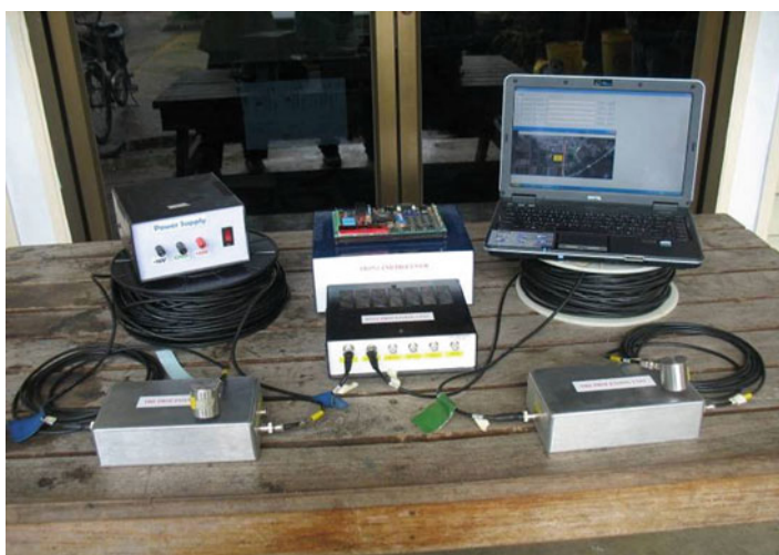
Fig. 10 Prototype of AE instrument for source location
