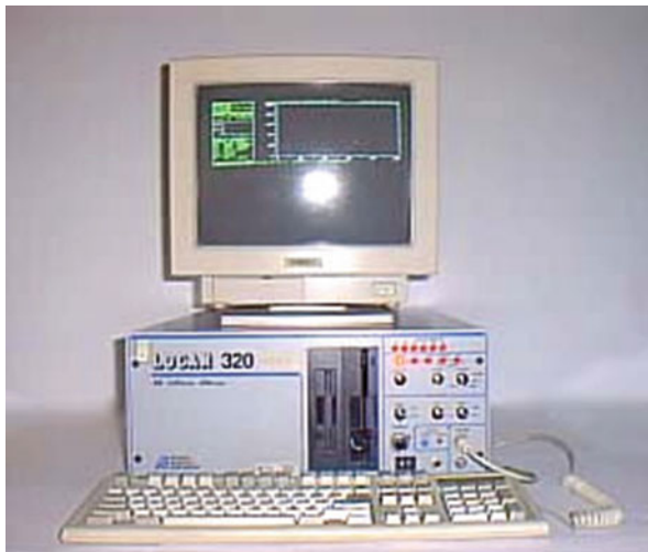
Fig. 8 First AE instrument in Thailand (PAC: LOCAN 320)
