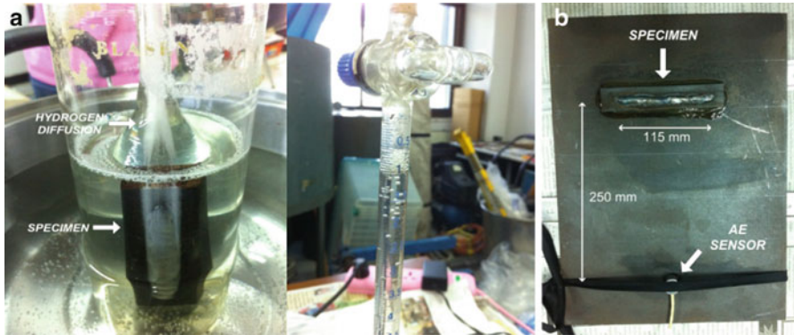
Fig. 2 (a) Apparatus of H_2 measurement, (b) specimen and sensor mounting on wave guide plate
