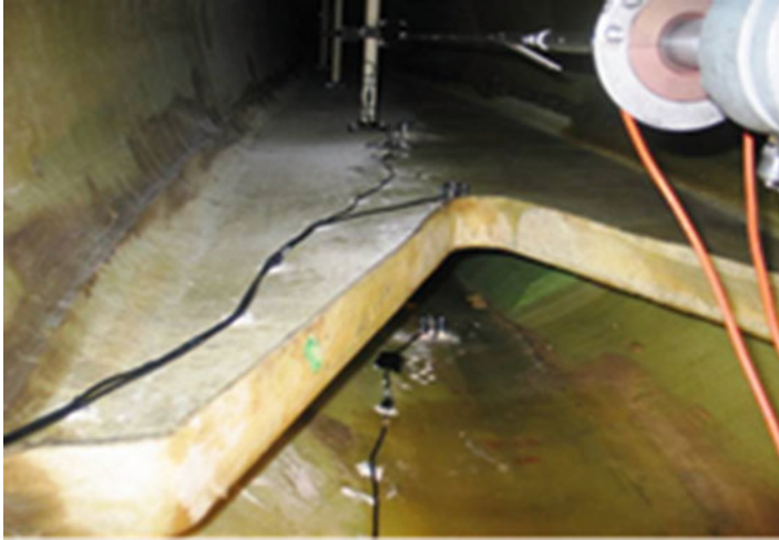
Fig. 4 Mounting of two AE sensors on the internal spar of a blade and one sensor on the inner surface of the trailing side of a blade [16]
