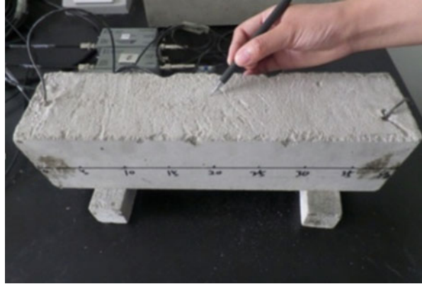
Fig. 4 Pencil lead broken at the concrete with embedded sensors
