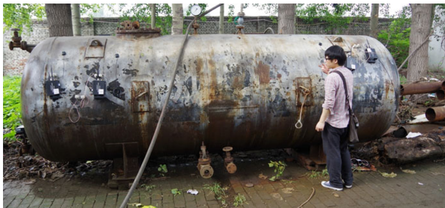
Fig. 7 The AE testing of LPG tank
