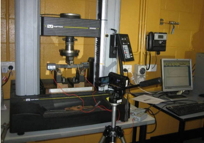
Fig. 1 Experimental setup for three-point bending tests
