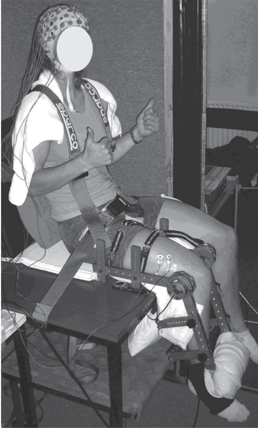
Fig. 17.7 Experimental setup for repeated isometric leg-extension protocol
