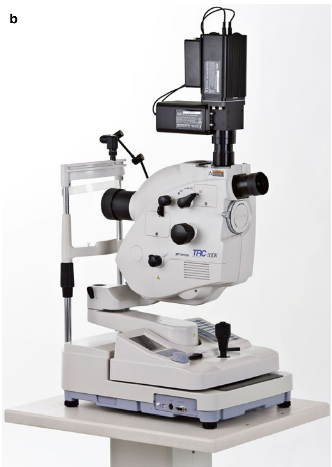
Figure IV.A-8 Pseudocolor retinal oximetry image (a) and spectrophotometric retinal oximeter (b). The oximetry image shows oxygen saturation in retinal vessels. The pseudocolor scale indicates oxygen saturation; red is 100 % saturation and violet is 0 %
