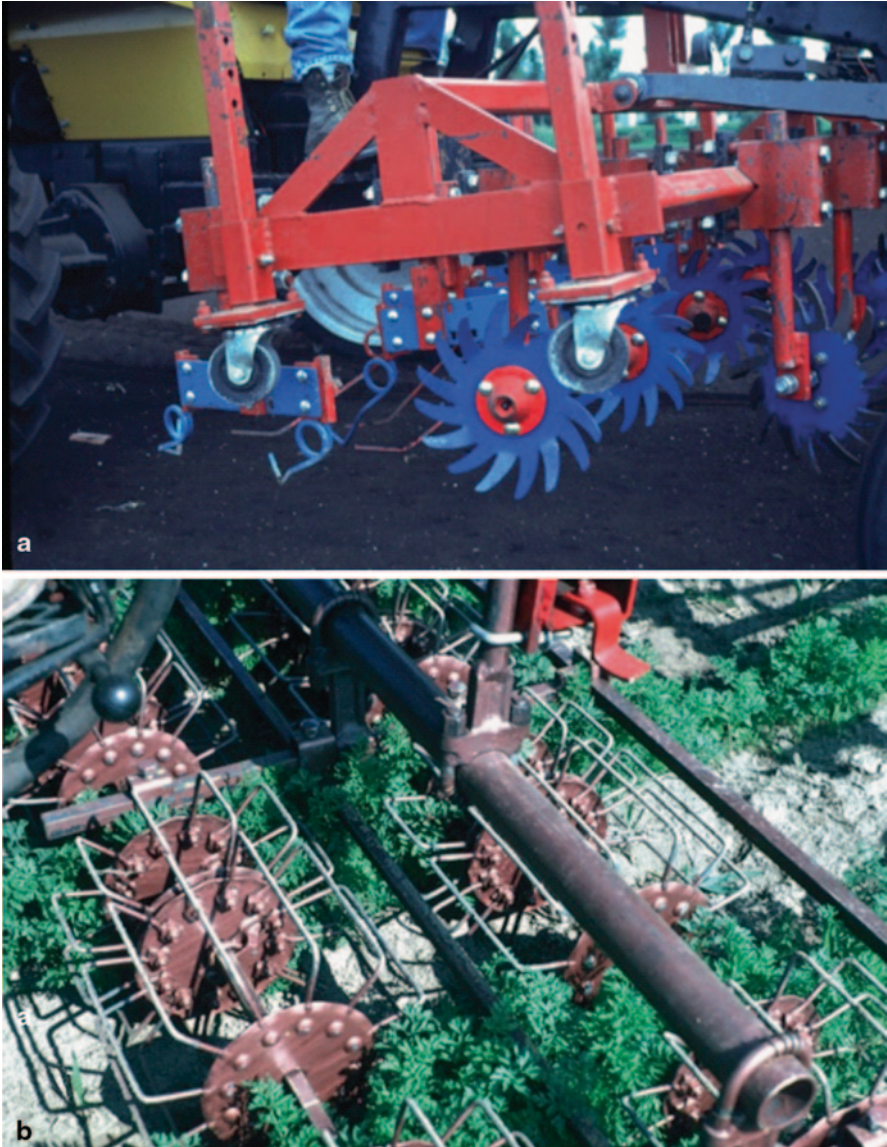
Fig. 11.1 (a) Torsion weeders with spiked discs, and (b) basket weeders are two types of mechanical weeders commonly used to control weeds in vegetable crops
