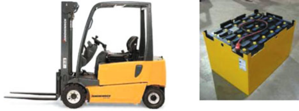
Fig. 19.1 A forklift and one of the batteries powering it. The cells in the battery can be seen in the figure
