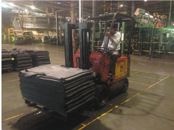
Fig. 19.3 Forklift moving a load of rubber sheets in a tyre manufacturing plant
