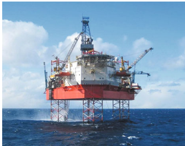
Fig. 13.2 The jack-up rig West Elara (©Seadrill)
