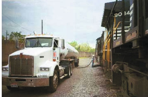
Fig. 2.3 A fueling truck refueling a locomotive (Source: http://www.bei-benedict.com/locomotive-refueling.php )
