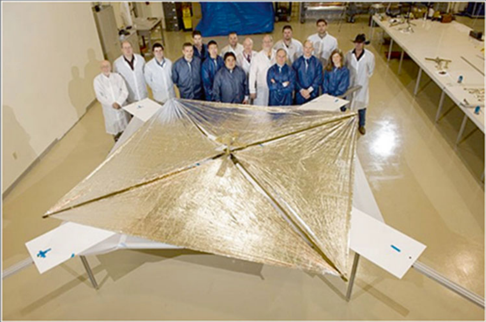
16.2 The NASA NanoSail D team celebrated the successful deployment of the sail prior to packaging for launch. The cubesat from which the sail deployed can be seen in the very center of the sail (Courtesy of NASA)
