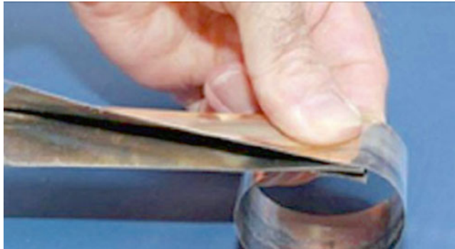
16.1 The coiled TRAC booms used on the NanoSail-D2 were developed by the US Air Force Research Laboratory (Courtesy of the US Air Force)
