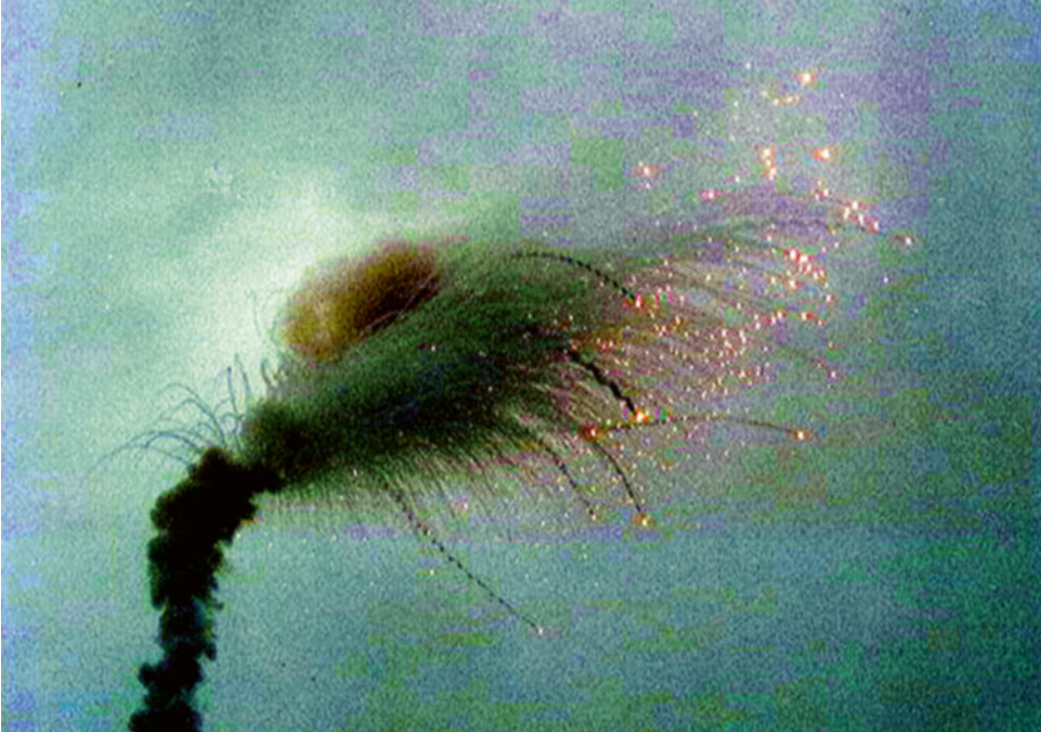
8.3 Ariane 501, the maiden flight of Europe's Ariane 5 launcher, veers off course and is destroyed by its automated destruct system (Courtesy of ESA)
