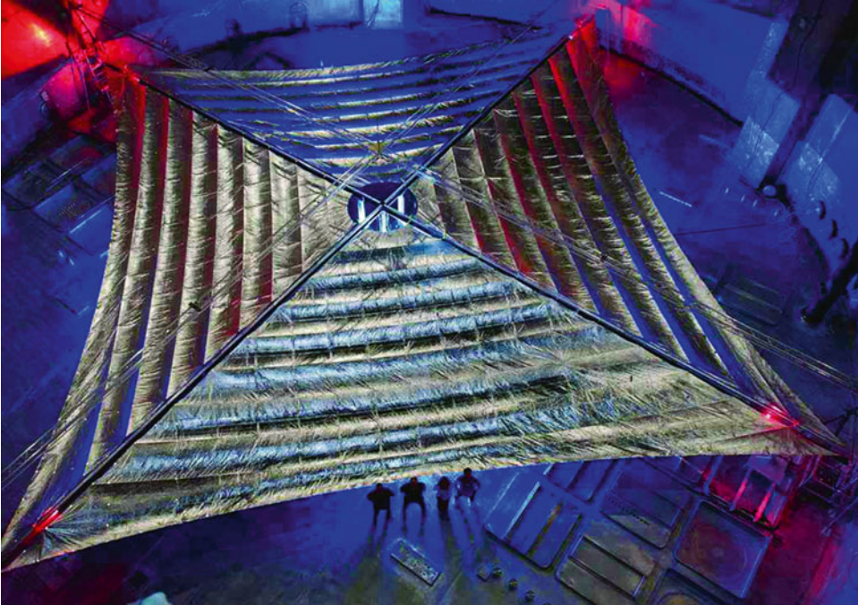
12.3 The L'Garde solar sail before vacuum testing at NASA's Plum Brook facility. The scale of the device can be appreciated by examining the relative size of the people in front of it (Courtesy of NASA)
