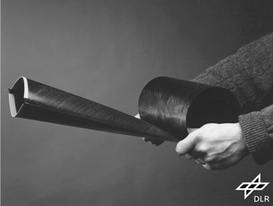
11.2 This rigid boom was used by DLR to deploy its solar sail during ground testing in 1999 (Courtesy of DLR)
