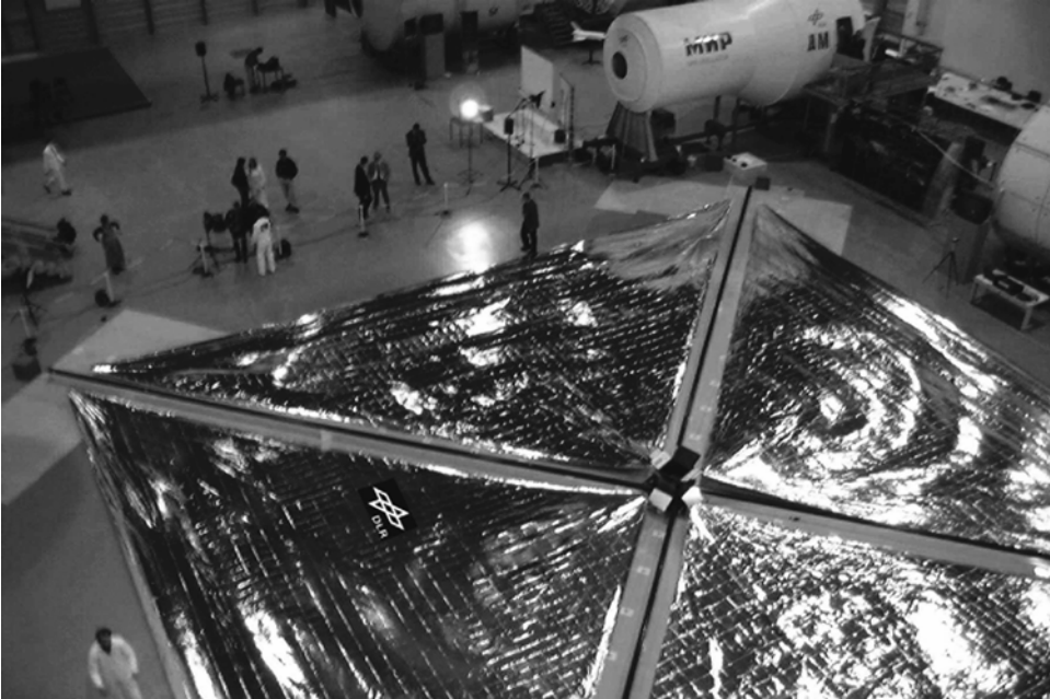
12.1 A photograph of the DLR solar sail ground demonstrator under full deployment (Courtesy of DLR)
