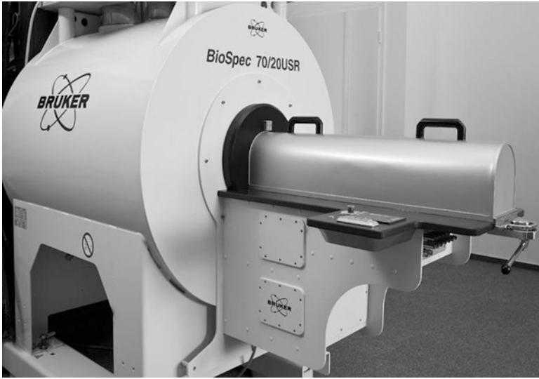
Fig. 7.7 Illustration showing a magnet with integral Faraday cage (courtesy of Bruker Biospin Ltd)
