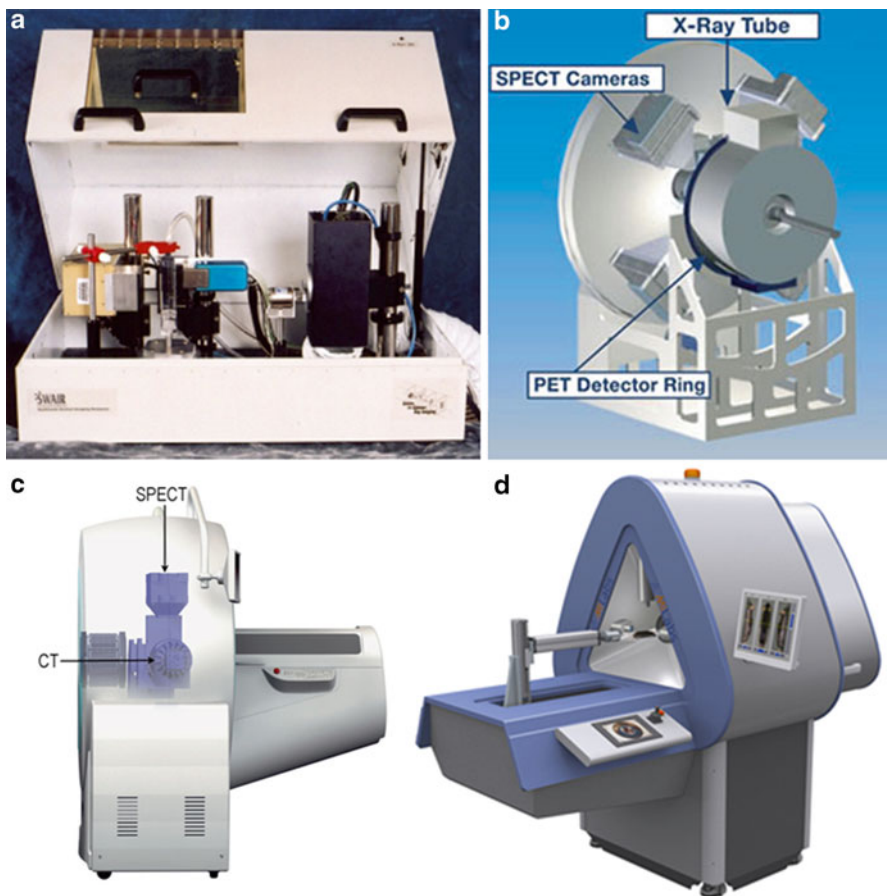
Fig. 12.3 Different flavors of preclinical SPECT/CT integration. (a) Compact box system that includes both small FOV X-ray CT and SPECT components from University of Arizona (Reprinted with permission from [28]). (b) An inside view drawing of Gamma Medica-Idea's FLEX Triumph™ gantry that shows the triple-modality (SPECT–CT–PET) configuration. (c) Another triple-modality configuration of a large gantry design with sufficient room around the scanner components (Siemens Inveon Multimodality gantry). (d) Docked SPECT/CT configuration–U-SPECT/CT from MILabs (figures of (b–d) are from product brochures)
