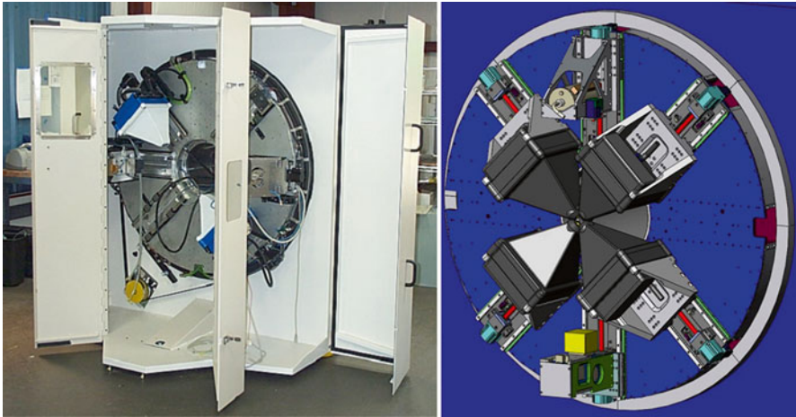
Fig. 12.2 UCSF MoHawk SPECT/CT scanner with two CZT-based pinhole SPECT cameras and X-ray cone-beam CT subsystem placed on a disk-gantry attached to a slip-ring ( left ). This system is designed to mount up to four pinhole/multipinhole CZT-based gamma cameras with a retractable in-plane microfocus CT ( right ) built on the same disk-gantry
