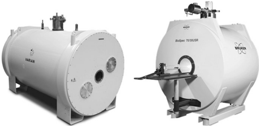
Fig. 7.5 Typical commercially available small animal MRI magnet systems. Left : A cryogenic unshielded ultra-high field 16.4 T small animal MRI magnet. For scale, the free bore diameter is 260 mm (courtesy of Varian Inc). Right : A 7 T, 300 mm bore ultra-shielded magnet with pulse-tube cryocooler for minimal helium boil-off (courtesy of Bruker Biospin Ltd)
