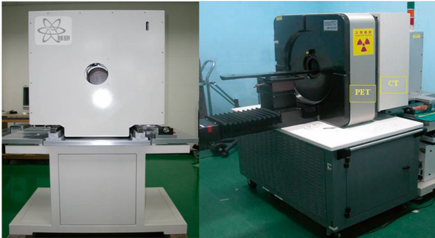
Fig. 13.4 Photo of a docking-type PET–CT system constructed by combining a custom built micro-CT scanner ( left panel ) with a commercially produced Siemens microPET R4, shown together in the right panel . Reprinted with permission from [33]
