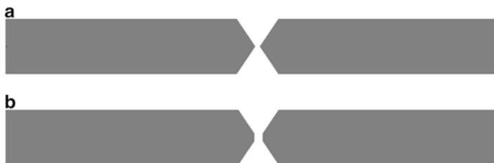
Fig. 4.5 Cross sections of pinhole collimators with (a) knife and (b) keel edges
