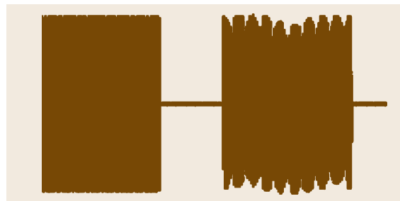
Fig. 15.5 Wave envelope of a major triad chord based on the just tuning scale followed by the same chord on the equal-tempered scale, with pronounced beats in the amplitude arising from the departures from harmonicity in the frequencies of the major third and perfect fifth
