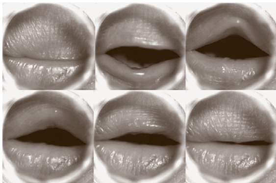
Fig. 15.103 High-speed photograph clips showing one cycle of lip vibration in a trombone mouthpiece
