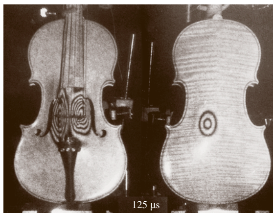
Fig. 27.12 Transient bending wave propagation in a violin body, 125 \mu\text{s} after impact start. The top of the bridge is impacted horizontally by a 5 mm steel ball at the end of a 30 cm-long pendulum (seen in the figure as a thin line). In the top plate a hill and a valley centered on the two bridge feet can be seen. In the back plate the fringes are centered at the soundpost, which rapidly transfers the impact from the bridge to the back of the violin (after [27.65], courtesy of AIP)
