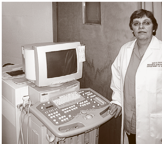
Fig. 21.62 Modern ultrasound imaging system. During the quarter century between 1975 and 2000, ultrasound systems retained the same exterior design, mounted on wheels, narrow enough to fit through a doorway, light enough that a sonographer could push the system, short enough so that a sonographer could see over the top and powered by a 1.5 kW outlet. To the right is the key to good ultrasound diagnosis, the well-trained, certified, experienced ultrasound examiner
