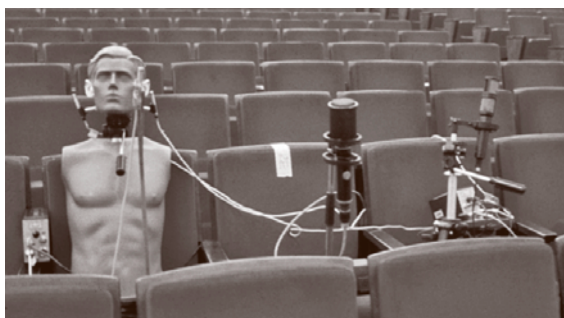
Fig. 9.12 A selection of microphones types used for recording impulse responses in rooms. From left: artificial head (with both internal and external microphones), sound field microphone (with four capsules for 3-D recordings of reflections) and a two-channel (stereo) microphone with omnidirectional and figure-of-eight capsules
