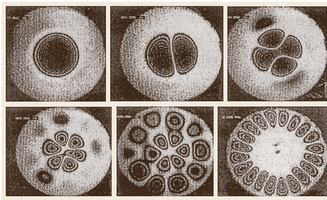
Fig. 28.7 Holographic interferograms of several vibrational modes in a Chinese gong. Note that some modes are mainly in the center of the gong, some in the outer portion, and some are global (after [28.19])
