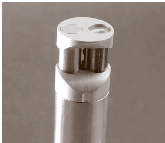
Fig. 25.18 A p - u sound intensity probe (by Microflow Technologies, The Netherlands)
