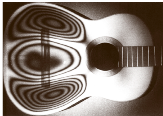
Fig. 27.3 Time-average interferogram of a guitar top plate vibrating at 505 Hz (Bolin guitar from 1969)
