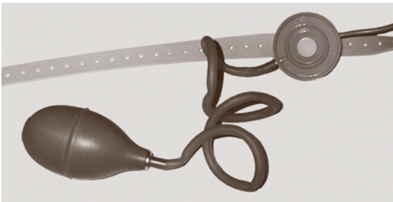
Fig. 21.3 Phono-cardiograph transducer. To avoid sounds and motions introduced by the examiner's hand on the chest, this phonocardiography transducer is fitted with a suction ring and elastic strap to secure the transducer element to the chest. Early echocardiographs had provision for amplifying and displaying the phono-cardiograph signals, which were filtered to display audible frequencies or infrasonic frequencies
