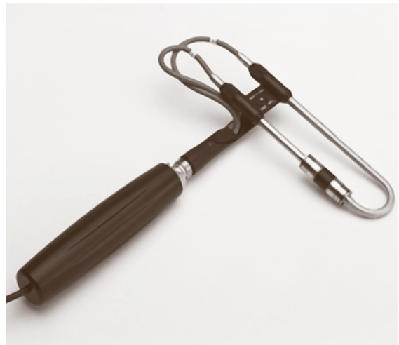
Fig. 25.7 Sound intensity probe with the microphones in the face-to-face configuration (Brüel & Kjær, Nærum)
