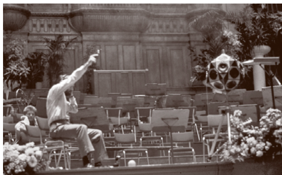
Fig. 9.11 Two types of omnidirectional sound sources for room acoustic measurements: blank pistol (in the raised hand of the seated person) and an omnidirectional loudspeaker (icosahedron with 20 units)
