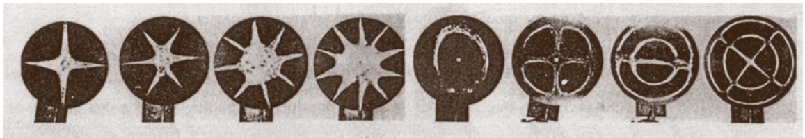
Fig. 2.1 Chladni patterns on a circular plate. The first four have two, three, four, and five nodal lines but no nodal circles; the second four have one or two nodal circles
