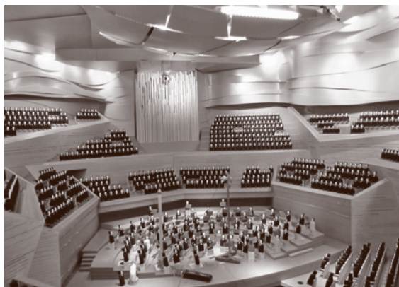
Fig. 9.15 A 1 : 10 scale model of the Danish Broadcasting concert hall in Ørestad, Copenhagen. The model is fitted with audience and orchestra (acoustic design by Nagata Acoustics, Japan)
