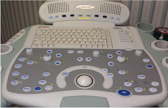
FIGURE 1.2 MyLab50. Panel of adjustable controls. (1) System on/off switch; (2) preset key allows the user to select from various menu items; (3) gain alters the amplification of the received signals in the image and by changing it the image brightness can be increased or decreased; (4) time gain compensation and depth gain compensation manual controls are useful to control the amount of amplification at different depths particularly when there is low attenuation of the image; (5) depth alters the image, and better view of the surrounding anatomy and less artifacts can be viewed in a large depth image; (6) the zoom function is used to magnify a region of the image on the screen; (7) the freeze function captures the image on the screen and allows to apply focus, measure, and save the image; (8) the calipers used to mark the area to be measured; (9) the image function saves the image in the system; (10) the clip function allows to take a video clip of various durations; (11) Doppler gain; (12) the start/end key saves the patient data and makes the system to be ready for the next study; (13) the archive review key permits the review of a specific exam and to save the entire session to an external drive, i.e., DVD and USB
