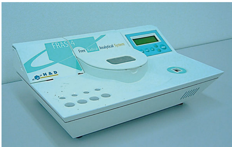
Fig. 8.1 Photographs of the FRAS4. The FRAS4 system was used under the following conditions: temperature 15–32 °C and humidity 20–80 %. The system is portable, being as small as 400 mm in width, 270 mm in depth, and 150 mm in height, and weighing as little as 4.0 kg. FRAS4 free radical analytical system 4
