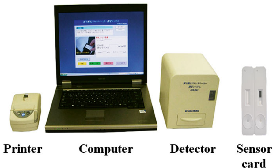
Fig. 8.3 Photographs of the automatic 8-oxodG analytical system, ICR-001. The ICR-001 system was used at a temperature of 18–30 °C and humidity of 30–80 %, and it had a width of 150 mm, depth of 160 mm, height of 170 mm, and weight of 2.8 kg. The sample-to-answer time was only 5 min for simultaneous detection of urinary creatinine and 8-oxodG concentrations. Test strips for 8-oxodG and creatinine are separately embedded in the sensor card. 8-oxodG; 8-oxo-7,8-dihydro-2'-deoxyguanosine
