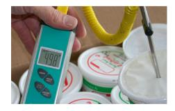
Fig. 7.3 Taking thermal readings of refrigerator contents using a digital thermometer (Source: CDC Public Health Image Library image # 13851/CDC/Amanda Mills)
