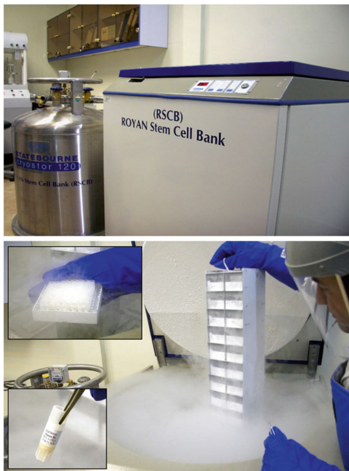
Fig. 12.2 Vapor phase nitrogen tank and its supply tank in RSCB
