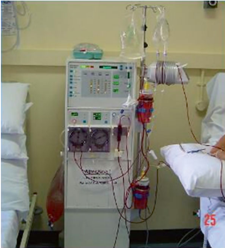
Fig. 15.3 The DALI machine that is used for lipid apheresis in patients with FH
