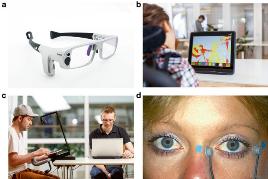
Fig. 2 Some examples of contemporary eye tracking equipment. From top to bottom : (a) Head-mounted mobile eye tracker in the form of eye tracking glasses (Courtesy: Tobii Technology); (b) table-based remote eye tracker (Courtesy: Tobii Technology); (c) eye tracking setup for mobile and personal devices (Courtesy: Tobii Technology); and (d) EOG (Source: Utah Medical School, http://webvision.med.utah.edu/ )
