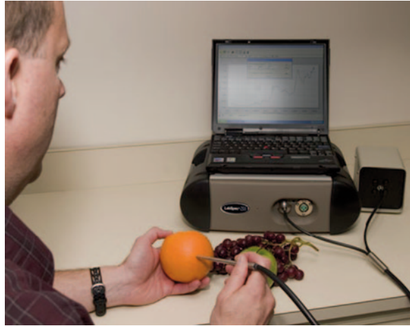
Fig. 4.6 A NIR (LabSpec) with bifurcated fibre optic probe for contact reflectance measurement
