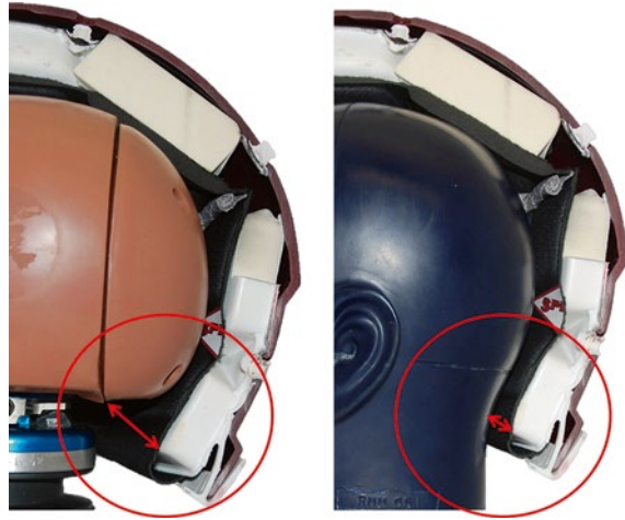
Fig. 7.12 The HIII and NOCSAE head forms with sectioned football helmet, illustrating the poor fit of the HIII head in the posterior head/neck region as compared to the NOCSAE head
