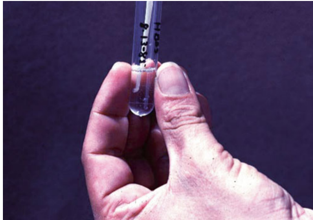
Fig. 18.7 Transferring of specimen to a test tube with glutaraldehyde fixative for EM
