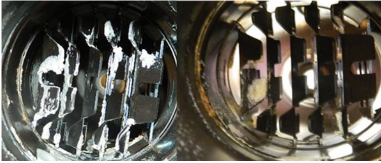
Fig. 15.32 Impact of calibration modifications on mixer depositing
