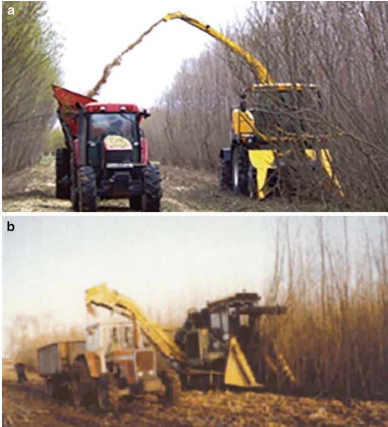
Fig. 5.29 Harvesting machinery for short rotation woody crops: (a) Case New Holland coppice harvester and chipper blowing chips into a tractor-pulled transfer bin. Adapted from [3]. (b) An Austoft cut-and-chip harvester chopping poplar. Adapted from [24]
