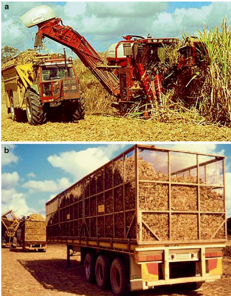
Fig. 5.35 (a) Sugar cane chopper-harvester in operation and (b) a truck trailer ready for long-distance travel. Adapted from [27]
