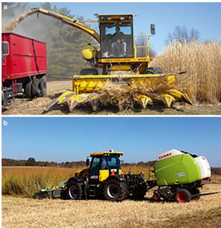
Fig. 5.25 (a) Self-propelled forage harvester chopping Miscanthus . (b) A single-pass machine that can mow and bale in a single pass
