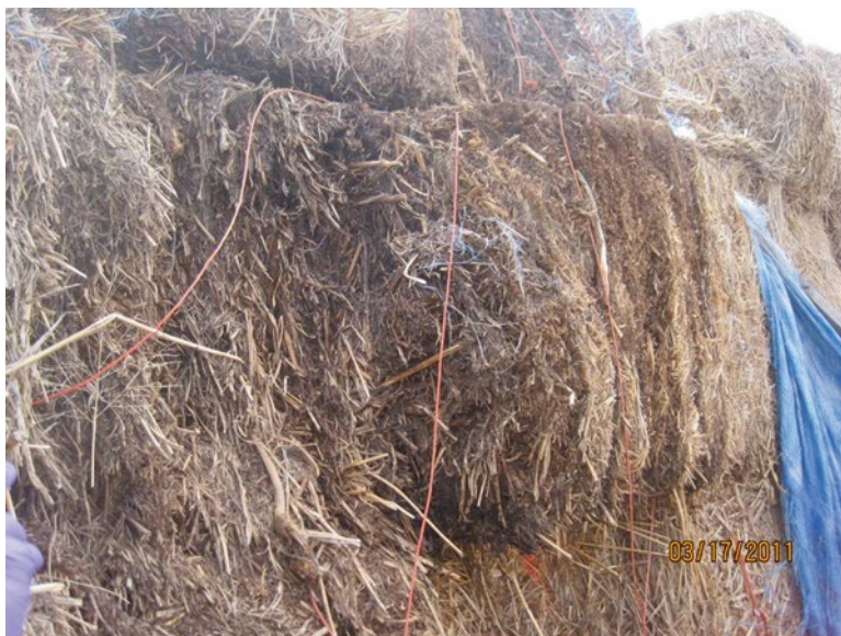
Fig. 7.10 Weathering of the outer layer of a switchgrass square bale in Pena, Illinois. Photograph courtesy of the Department of Agricultural and Biological Engineering of the University of Illinois
