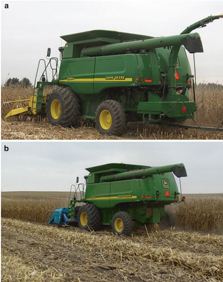
Fig. 5.39 (a) Combine harvester configured to harvest corn stover in a single pass using a precision-cut stover processor. (b) Combine harvester configured to harvest stover in two passes by forming stover windrows during grain harvest. Adapted from [36]
