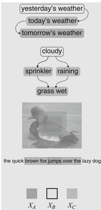
Graphical Models, Fig. 1 Some examples of conditional independence; we say that X_A and X_B are conditionally independent , given X_C , or more compactly X_A \perp X_B \mid X_C
