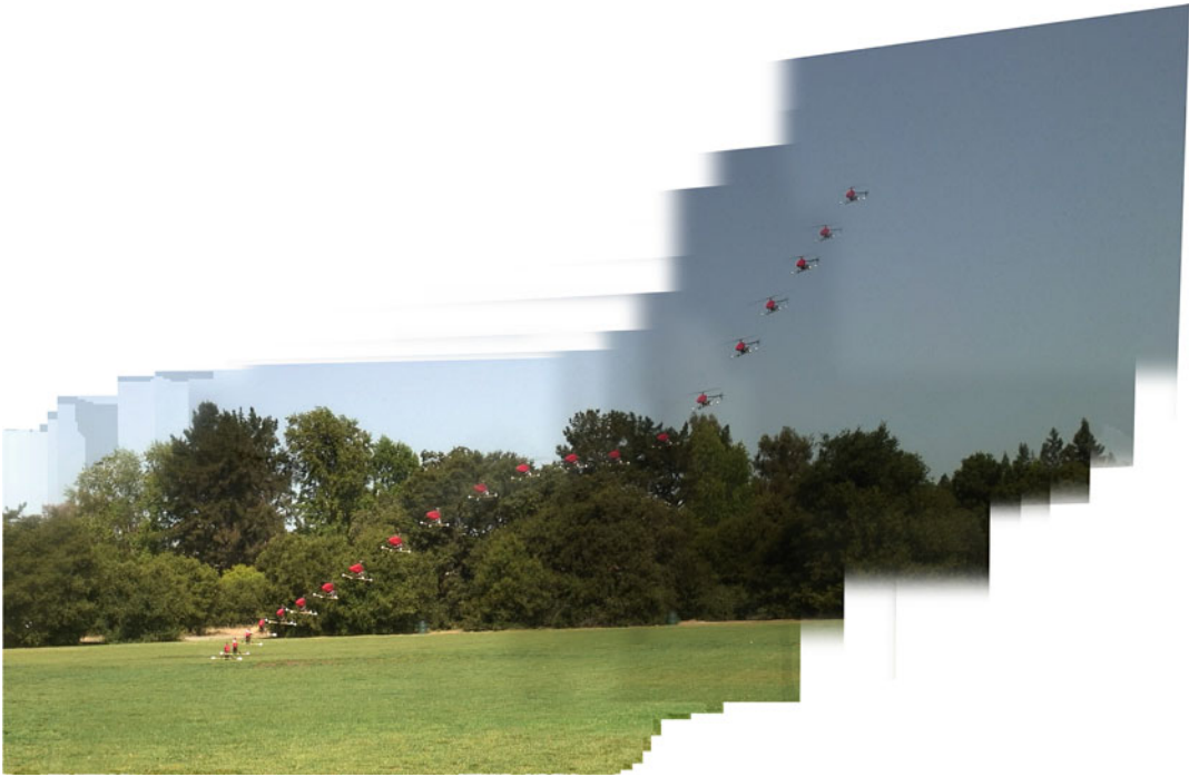
Autonomous Helicopter Flight Using Reinforcement Learning, Fig. 4 Superimposed sequence of images of autonomous autorotation landings (from Abbeel et al. 2008)
