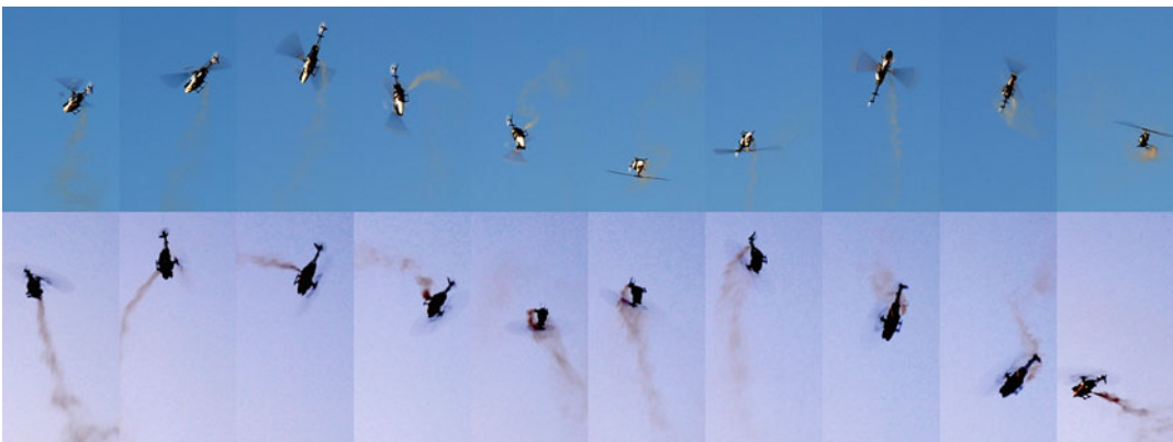
Autonomous Helicopter Flight Using Reinforcement Learning, Fig. 2 Snapshots of an autonomous helicopter performing in-place flips and rolls
