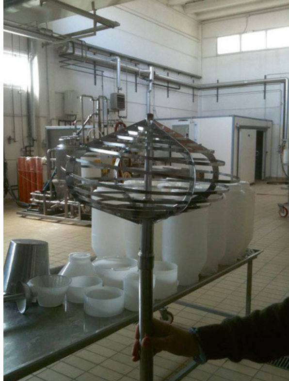
Fig. 8.2 A spino used to break the curd during the manufacture of certain Italian cheeses
