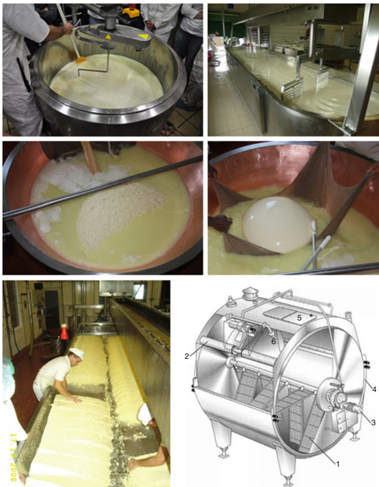
Fig. 2.4 Examples of vats used for cheesemaking
