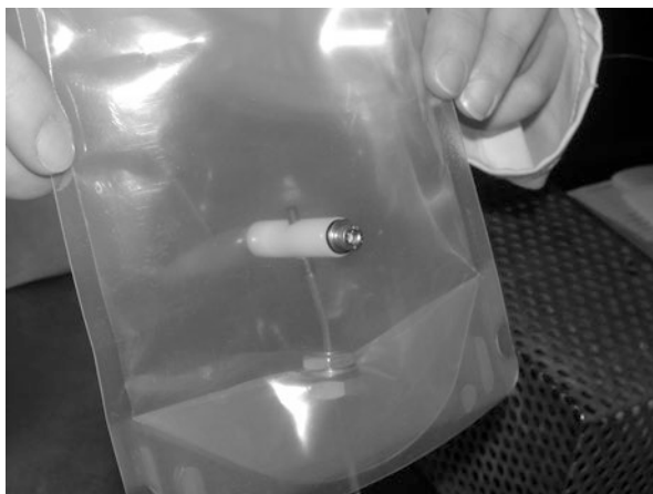
Fig. 10.3 Thermocouple held in place in retortable pouch
