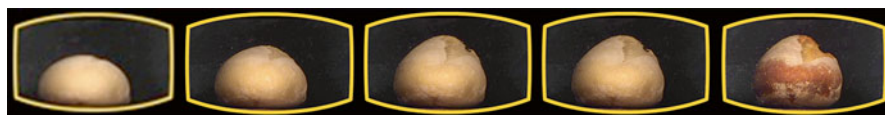
Fig. 11.5 Baking without steam at T_{\text{sole}}=260 °C, T_{\text{vault}}=245 °C at five observation times (1, 4, 6, 8, 27 min)
