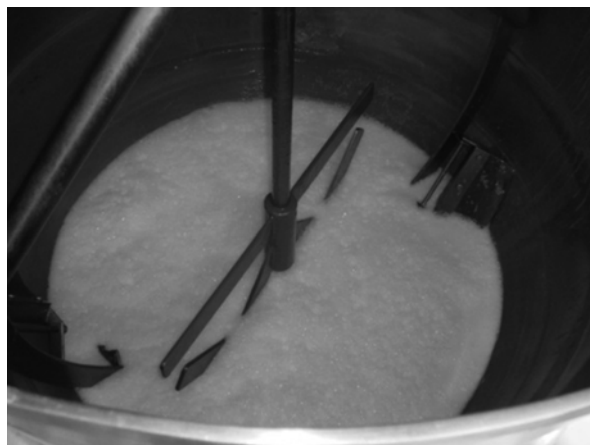
Fig. 9.6 Internal view of jam pail and its stirring system while producing DDL
