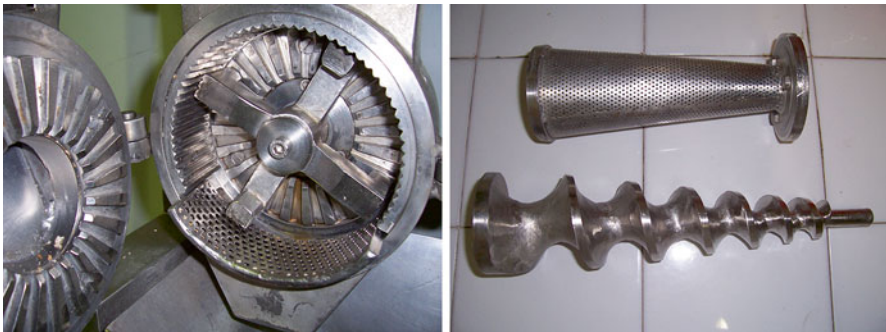
Fig. 28.2 Detail of a hammer mill (left) and a worm gear and its filter (right) used in the production of horchata
