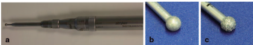
Fig. 14.17 a Neurosurgical grinding device and diamond wheel with b 25/30 ANSI mesh (711 FEPA), and c 200/230 ANSI mesh (76 FEPA) diamond grit
