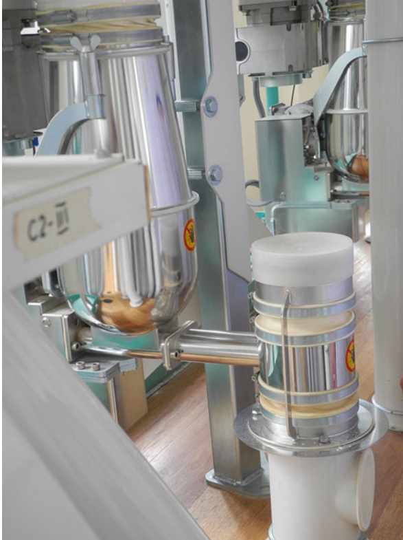
Large-scale mill dosifier. Project Healthy Children 2011
