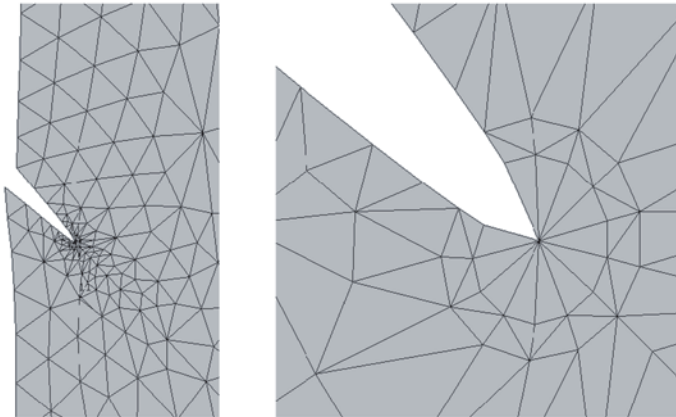
Fig. 8.72 Deformed shape of the crack ( left ) and the deformed shape in the vicinity of the crack tip ( right )
