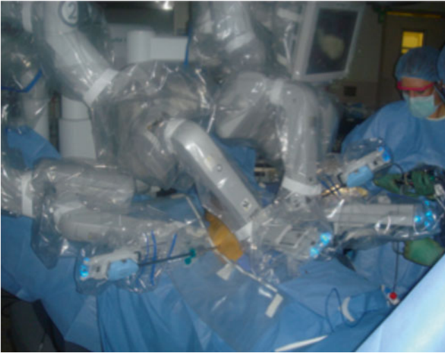
Fig. 4.6 Patient side cart. For Fig. 4.6: provided here exclusively for promotion and/or media coverage of Intuitive Surgical and its products. This notification serves as an authorization for publications to make duplicate copies of the available high-resolution scans for editorial use only (© 2014 Intuitive Surgical, Inc. All people depicted unless otherwise noted are models)
