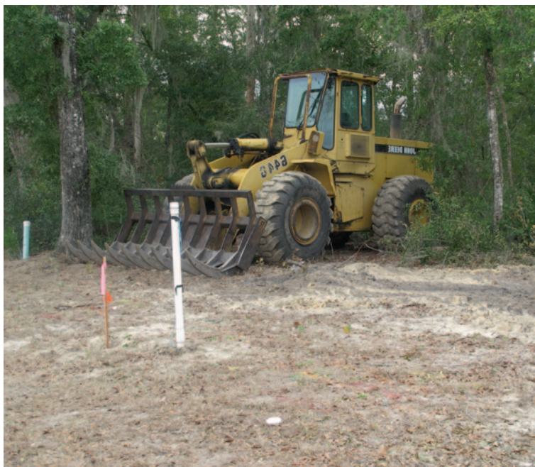
Fig 13.2 Earthwork machines can have large impacts on open spaces conserved for biodiversity. In Florida, contractors typically park their vehicles in forested areas to escape the heat. Running or parking earthwork machines under trees has the unintended consequence of killing the trees and even compacting the soil to the point where it reduces percolation rates of stormwater running off of impervious surfaces. (Source: Jeanette Hostetler)
