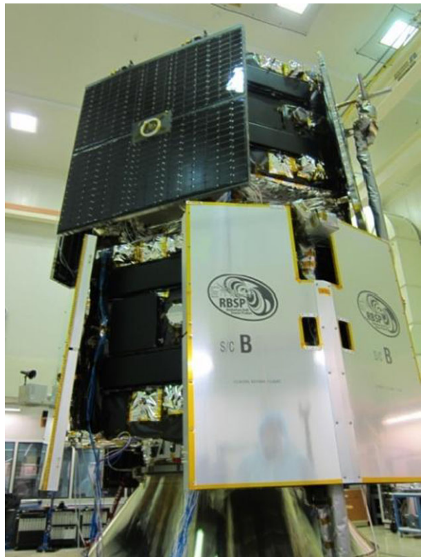
Fig. 37 RBSP observatory stacked in launch configuration for system test (Photo: Lee Hobson, JHU/APL)
