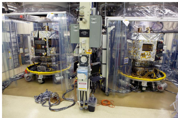
Fig. 40 RBSP Observatories A and B side by side prepared to lift into thermal vacuum chambers at JHU/APL (Photo: Ed Whitman, JHU/APL)
