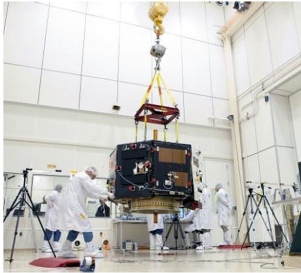
Fig. 15 Observatory magnetic swing test configuration
