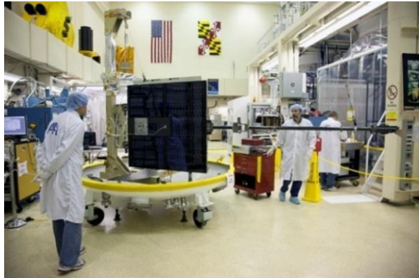
Fig. 39 In-air deployment test of solar array wing (Photo: Ed Whitman, JHU/APL)
