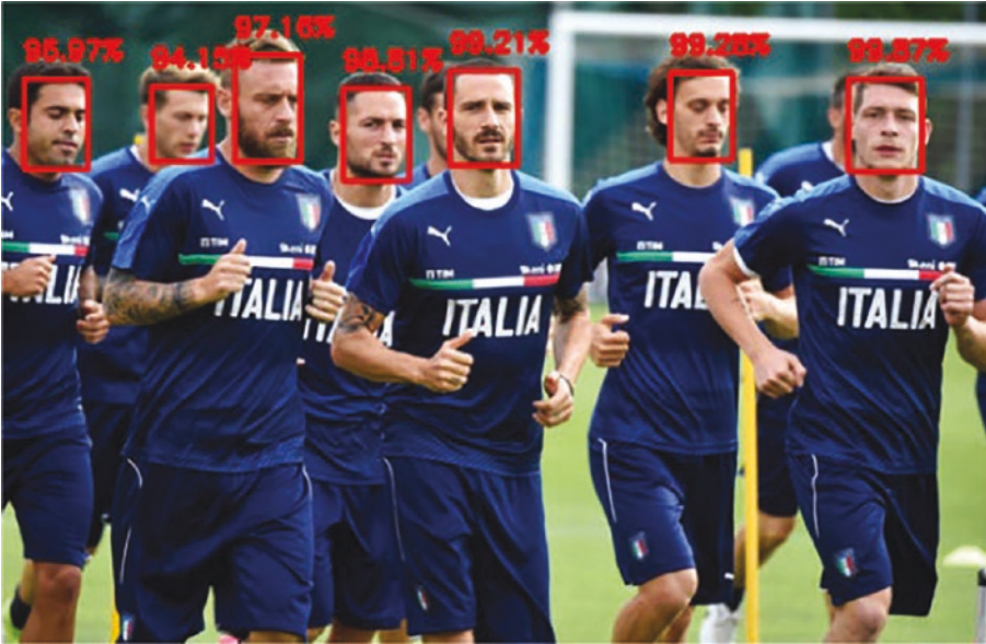
Figure 14-18. The faces of the national football players have all been accurately recognized
