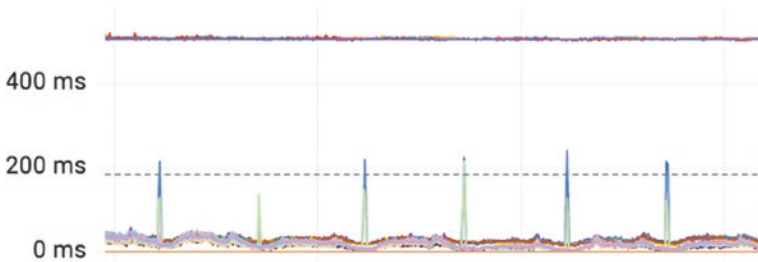
Figure 10-9. Spikes in the time it takes the rogue broker (represented by the green line) to serve fetch requests from the consumers
