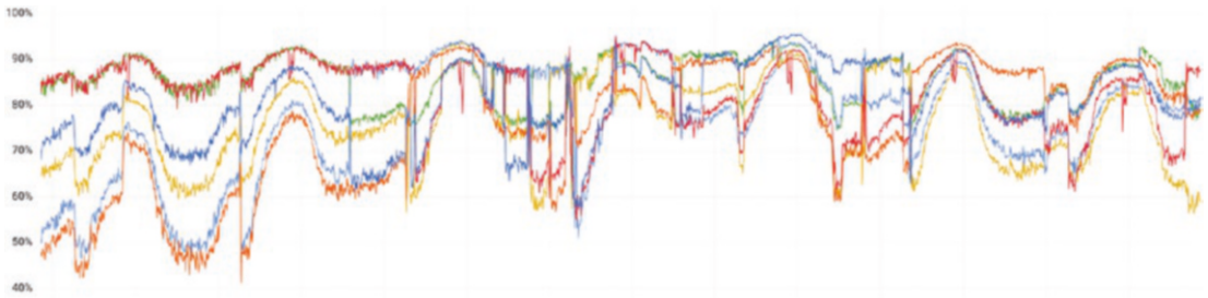
Figure 10-6. Drops of network processor idle% time (which is equivalent to spikes in their busy%) in all brokers but especially in the rogue broker (represented by the orange line)
