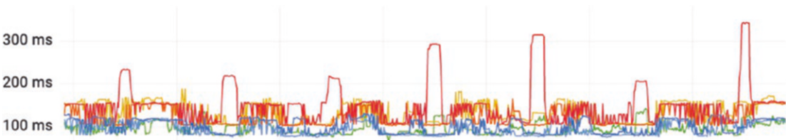
Figure 10-10. Spikes in the log flush rate in the rogue broker (represented by the red line)
