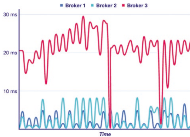
Figure 7-22. Wait time for write operations on the disks of each broker during peak traffic time
