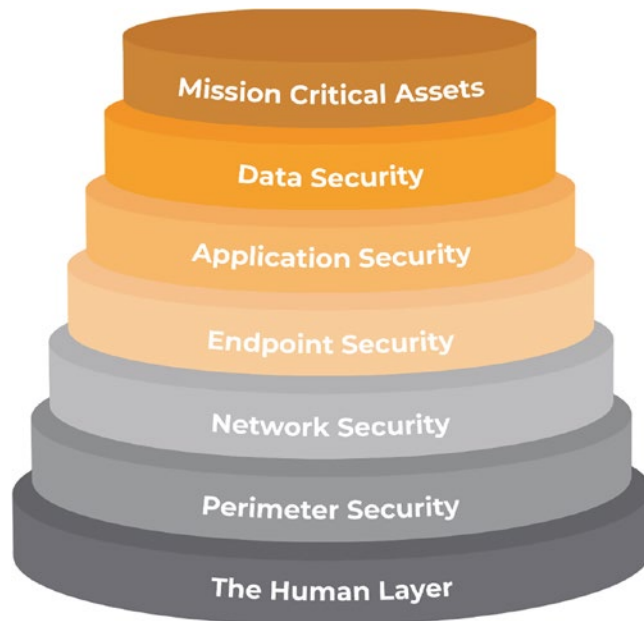
Figure 4-12. Layered security architecture
