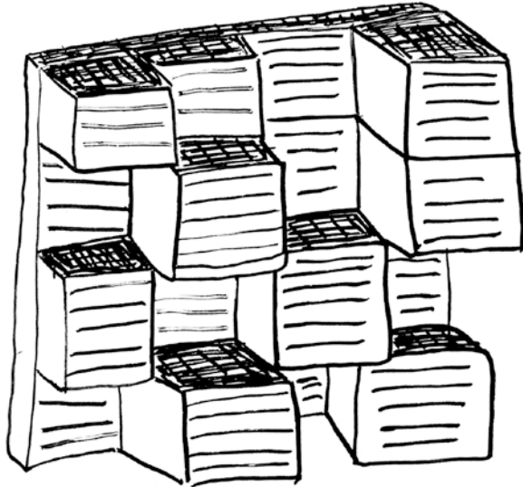
Figure 5-5. A section of a diffuser
